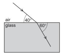
The angle between the ray and the edge of the glass block is  $40^{\circ}$  in the air and  $60^{\circ}$  in the glass.
