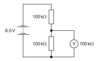
A voltmeter of resistance  $100\,k\Omega$  is connected across one of the resistors.
