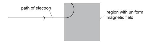
In the magnetic field, the electron follows a semi-circular path of diameter 0.0700 m.
