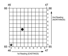
To give the six-figure grid reference, first identify the grid square, in this case 4665. The third figure is obtained by dividing the space between grid lines 46 and 47 into ten equal parts. Similarly, the sixth figure is obtained by a division of the gap between northings 65 and 66. This results in a grid reference of 463654 for the dot and 460650 for the star. Please note that the first tenth is 0 and the last tenth is 9 in the divided grid square.
