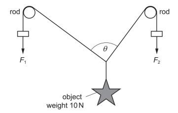
The object is held in equilibrium by the forces  $F_1$  and  $F_2$ . The object weighs 10 N. There is negligible friction between the rods and cords.
