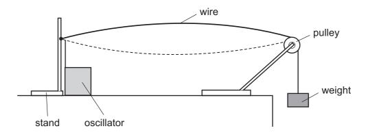
An oscillator is attached to the wire near the fixed end. A stationary wave with one loop is produced. The frequency of the oscillator is f.
